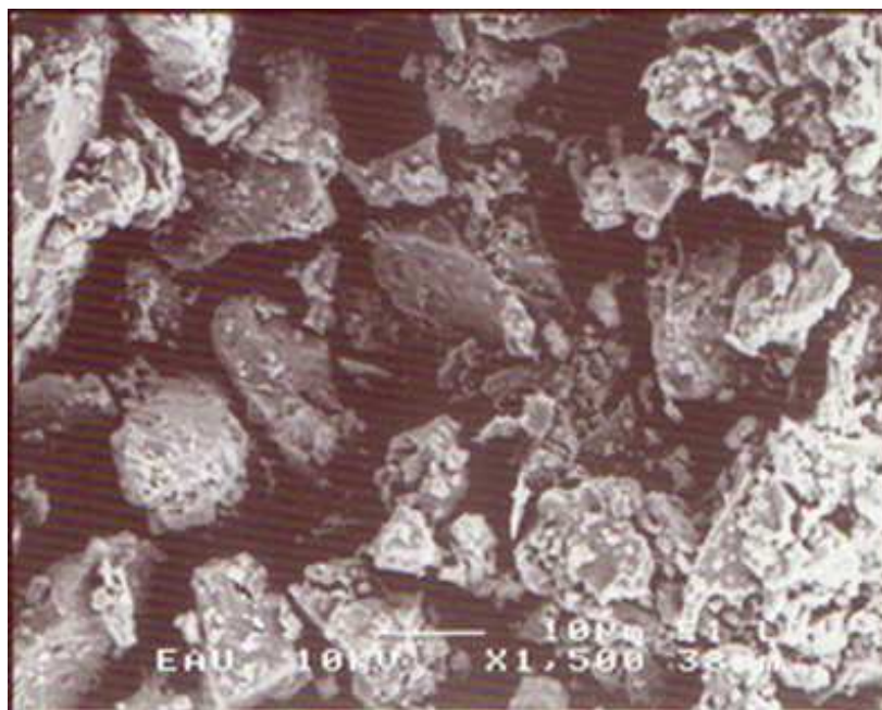
Figure 2. SEM photograph of the chalcopyrite concentrate
