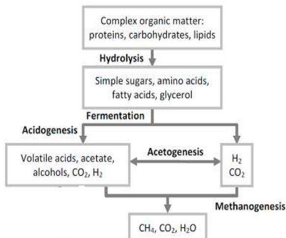
**Figure 1.** Anaerobic Methane Production
