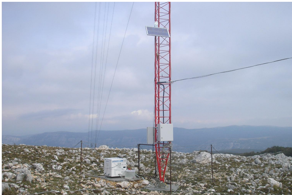
Figure 3. The measurement site Hrgud, LIDAR (left) mast (right)
