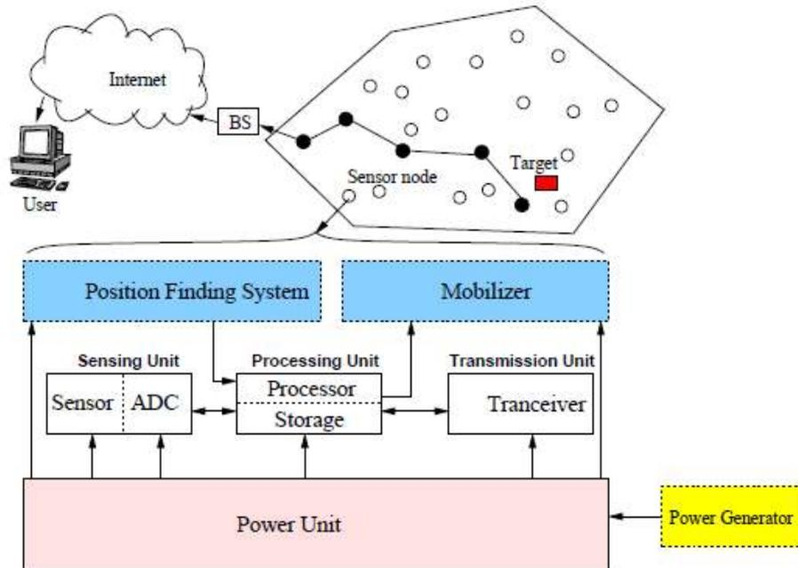
Figure 1. The components of a sensor node [1]
