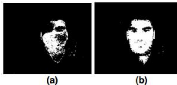
Figure 3. (a) detection of the areas with skin color using RGB code technique (b) detection of the areas with skin color using YCbCr code technique.
